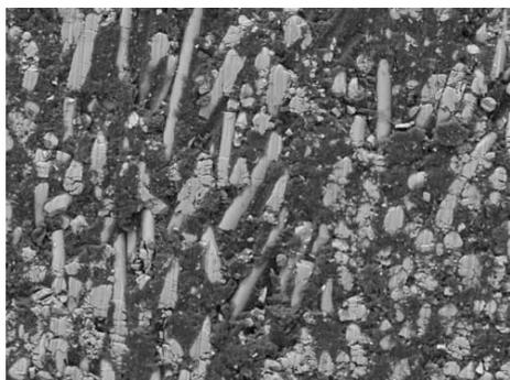
**Fig. 1** SEM micrograph of the cross section of a PF moulding compound. Glass fibres (light colour) with an average diameter 12  $\mu\text{m}$  are seen in various orientations in the matrix of cured novolac resin and fine-grain filler
