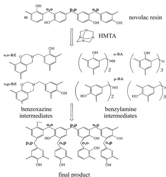
**Scheme 1** Polycondensation reaction between novolac resin and HMTA
