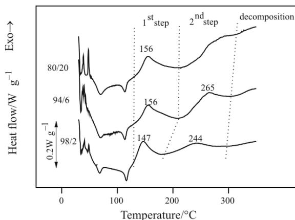
**Fig. 5** Influence of HMTA content on the curing reaction in an argon atmosphere (pressure 50 bars, heating rate 10 K min<sup>-1</sup>)
