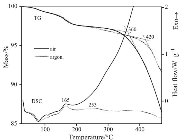
Fig. 6 TG and DSC curves of a sample with N/HMTA=98/2 under air and argon atmospheres (normal pressure)
