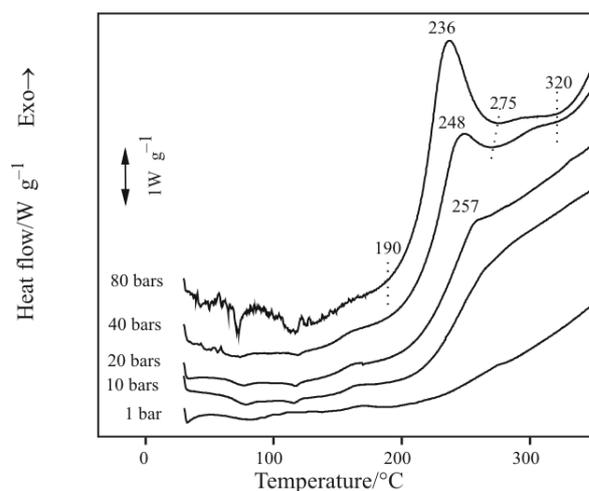
**Fig. 3** DSC curves of a sample with N/HMTA=80/20 under an air atmosphere; heating rate  $20 \text{ K min}^{-1}$
