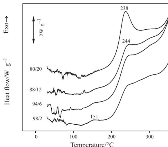
**Fig. 4** Influence of HMTA content on the shape of a DSC curve under an air atmosphere (pressure 80 bars)
