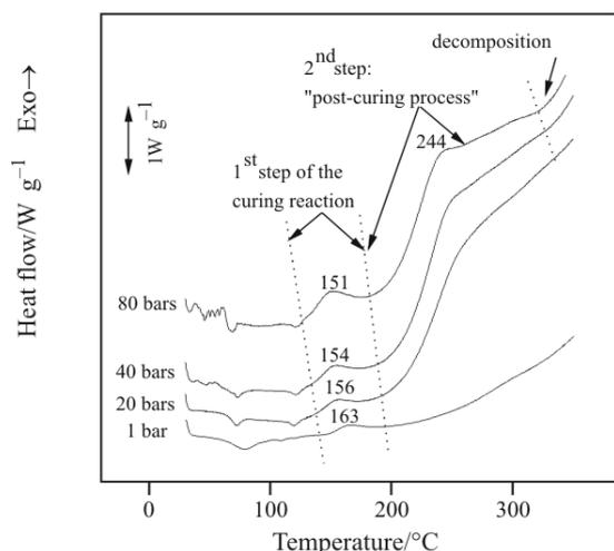
**Fig. 2** Influence of pressure on the shape of the DSC curve for a sample with N/HMTA=98/2 under an air atmosphere. The heating rate was  $20 \text{ K min}^{-1}$
