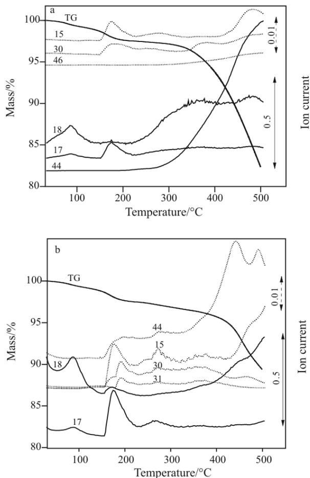
Fig. 7 TG-MS curve of a sample with N/HMTA=98/2 under a – air and b – argon atmosphere
